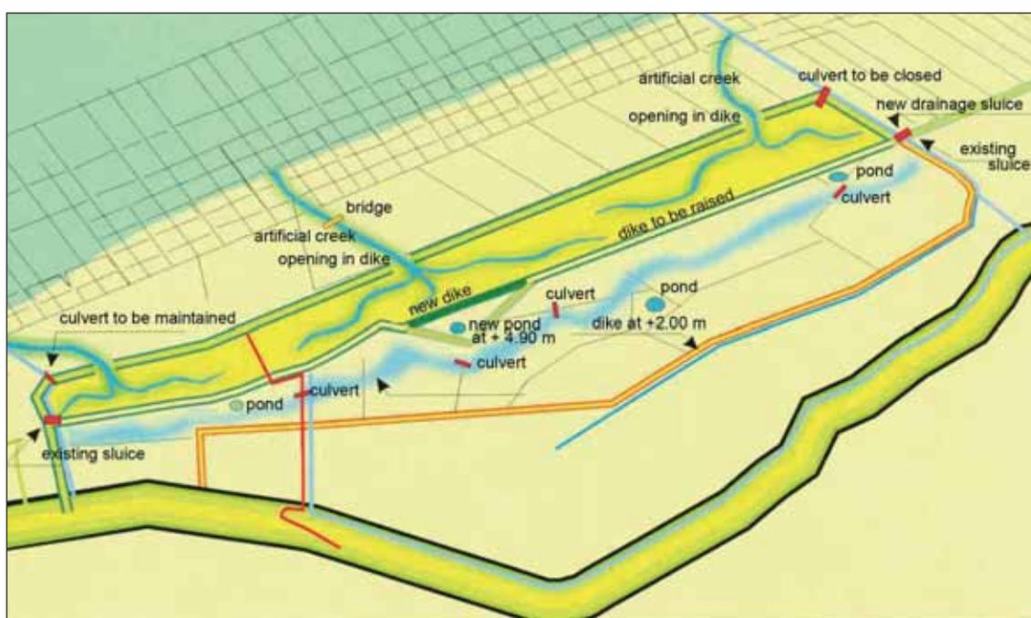
Figure 2. Plan for the experimental saltmarsh in Noard-Fryslân Bûtendyks undertaken by It Fryske Gea. After a drawing by Oranjewoud.
