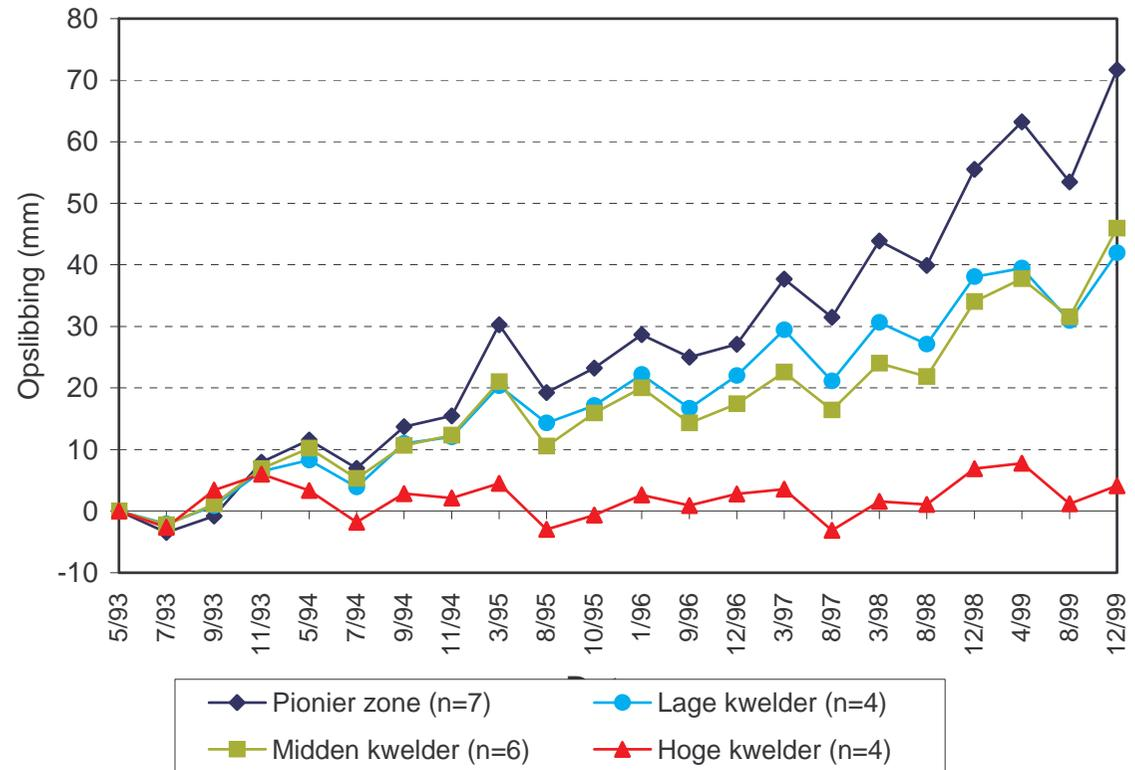
Results of the annual measurements using the "sedimentation-erosion bar method" (transect 3). In the lower zone (pink line) sedimentation is highest (12 mm/yr), close to the dunes (red line), sedimentation only occurs during severe storms.
