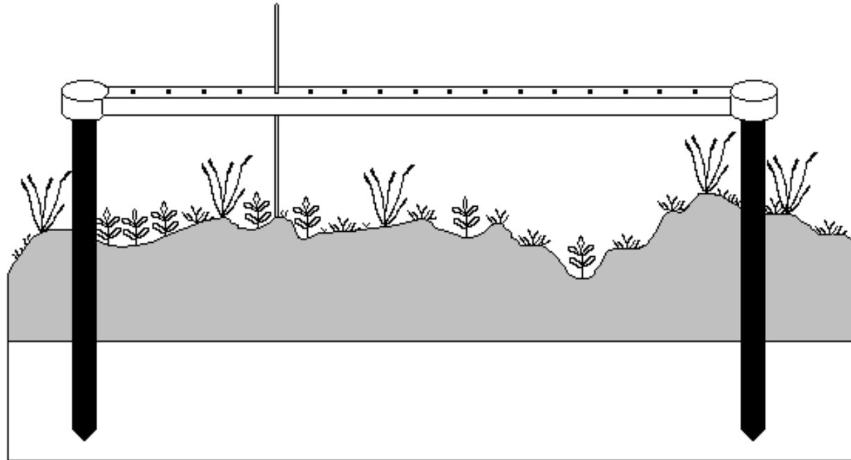
*The "Sedimentation – Erosion Bar method" (SEB) is used to measure annual sedimentation – erosion.*
