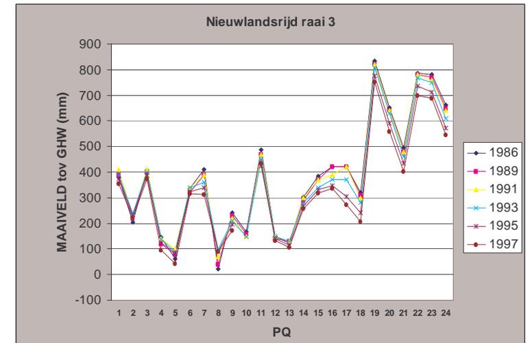
The development of the ground level in the transects 3 and 9 in the period 1986 to 1999. The subsidence of 15 cm (transect 9) at the edge of the marsh fully is fully compensated by annual sedimentation. At some distance from the sea and creeks, less silt is available and compensation is partial.
